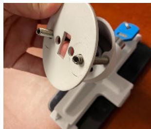
3. Align the studs with the holes in the fixture. Feed the charging cable up through the base of the Scorpion.
