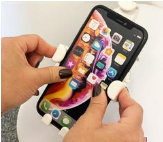
7. Once device is centered, press on push buttons to tighten the legs to the device.
