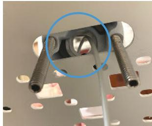
4. Feed the charger through the under counter plate. Next, tighten the wingnuts on both sides until secure. (There is a notch in the base, set the cable there)
