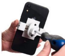
10. Place the installed device into the receiver. Press the lock in to secure. Scorpion should now be locked into place.
