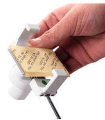
3. Place the device into the Scorpion and ensure that the leveling plate is aligned in the center of the device.
