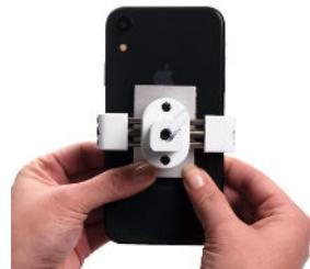
5. Tighten the side legs of the Scorpion until they slightly touch the side of the device by inserting the blue key into the axle (green dot side) and rotate clockwise.
