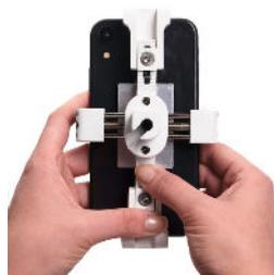
6. Tighten the side legs of the Scorpion until they slightly touch the side of the device by inserting the blue key into the axle (green stickers side) and rotating clockwise.
