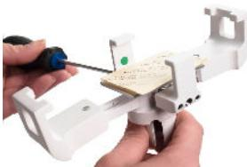
4. Place the device into the Scorpion and ensure that the leveling plate is aligned in the center of the device.
