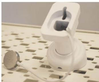
3. Take the top, and use the security key on the axle of the Scorpion and turn counter clockwise to ensure that the legs are fully extended. Once the legs are fully extended, insert the charging puck.
