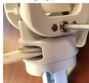
4. Place the watch into the Scorpion, and use the security key to tighten the legs to the watch, by turning clockwise until the legs are snug against the watch.
