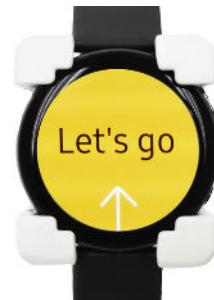
6. Tighten the side legs of the Scorpion until they slightly touch the side of the device by inserting the security key into the axle and rotate clockwise.
