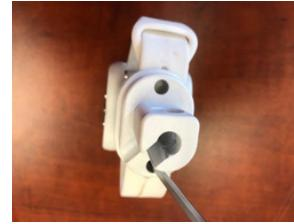
**NOTE:** Alternate 3 turns per stud until plate is raised
