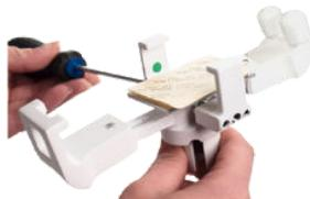
4. Place the device into the Scorpion and ensure that the leveling plate is aligned in the center of the device.
