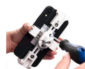
**NOTE:** 3 turns and switch until plate is raised
