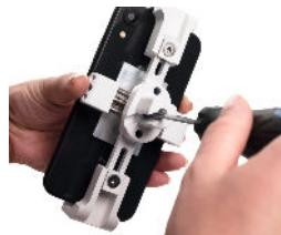
12. Place the installed device into the receiver. Press the lock in to secure. Scorpion should now be locked into place.
